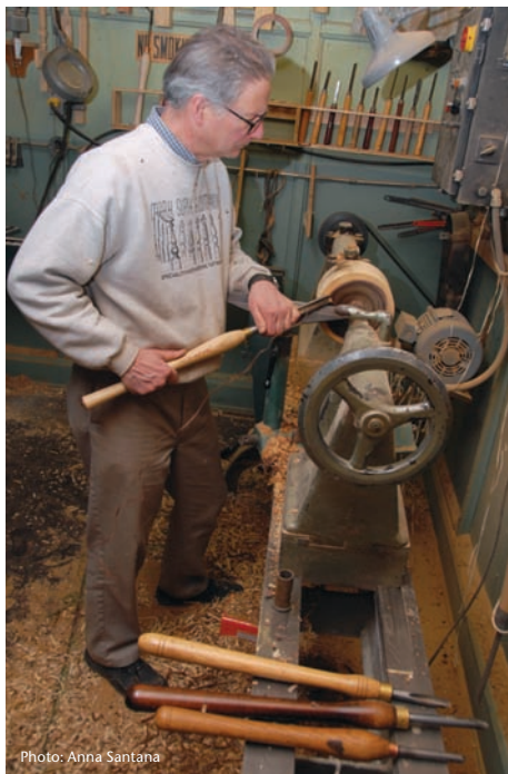
Vessel turning offers Mark the opportunity to create without specifications. The beefy tailstock here sits atop a 1920s American (brand) lathe.
