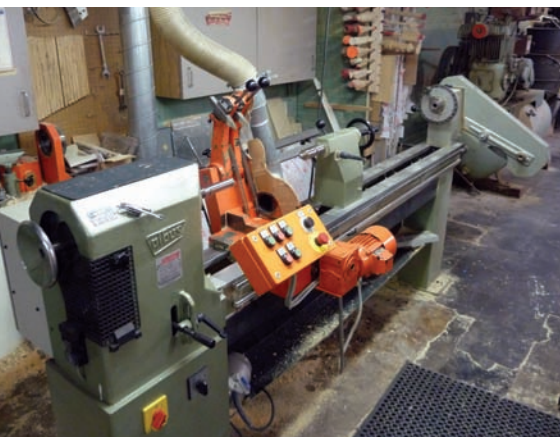
The Hapfo copy lathe has ultimately paid big returns on a dicey investment through its speed, accuracy, and capacity to produce high volumes, as well as fluting and rope molding.
