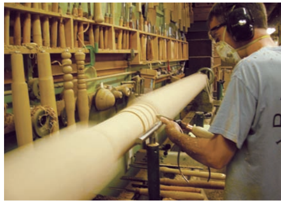
(Left) John Supik takes advantage of the generous span afforded by one of two salvaged long-bed lathes in the shop.
